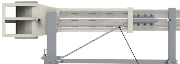
Anchor cable is fed inside through the MFLEAT feeder chute.
